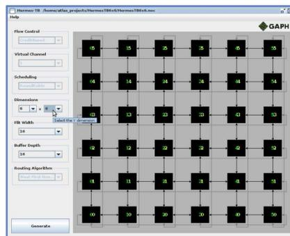
FIGURE 1: NoC Generation GUI.
